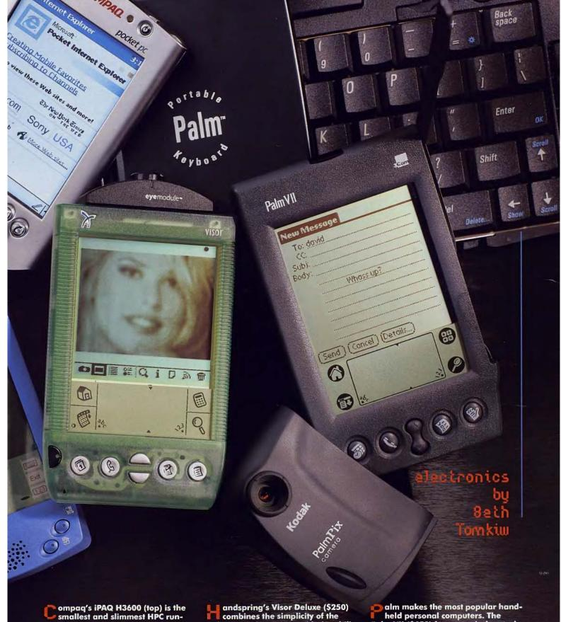
ompaq's iPAQ H3600 (top) is the smallest and slimmest HPC running the Windows-based operating system. The iPAQ is about the size of a calculator and is powered by a 206 MHz Intel Strong ARM processor and 32 megs of RAM. It syncs with your PC via a USB connection and offers all the capabilities of its competition, including a built-in voice recorder (so you can attach voice messages to e-mail) and the ability to play digital music. Price: about \$500.
